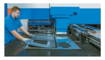
Parts over  $500 \times 500 \text{ mm}$  are picked from the table.
