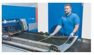
Skeletons can be removed from either side of the machine.
