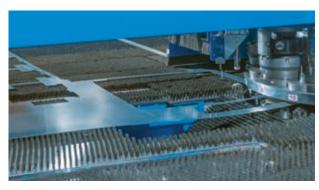
Punched parts up to  $500 \times 500$  mm are dropped through the door in front of the turret for separate sorting.
