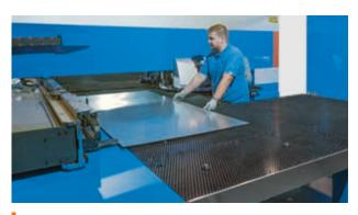
Larger sheets are positioned against the first and second loading pin.
