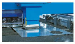
Laser cut parts up to  $500 \times 500 \text{ mm}$  (machine size 1225) or  $300 \times 400 \text{ mm}$  and  $800 \times 800 \text{ mm}$  (machine size 1530) are dropped through the door in the table onto conveyor below.
