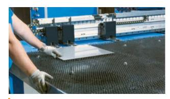
Smaller sheets are positioned against the third and fourth loading pin.
