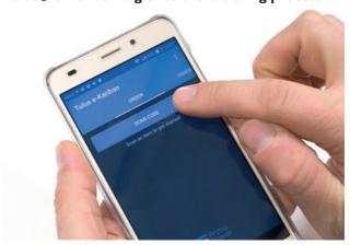
Tulus e-Kanban can be used for all part ordering processes, not only sheet metal parts. Part's metadata is used to determine where the order is placed, how large is the batch size, storage location, etc. Order can go either to ERP or directly to Tulus® Power Processing order management. Operators no longer need to look for paper orders because orders are entered digitally directly to where they are intended.
