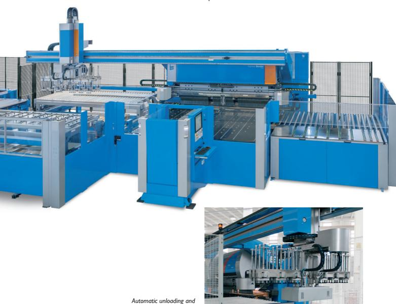
stacking add unmanned production capacity
