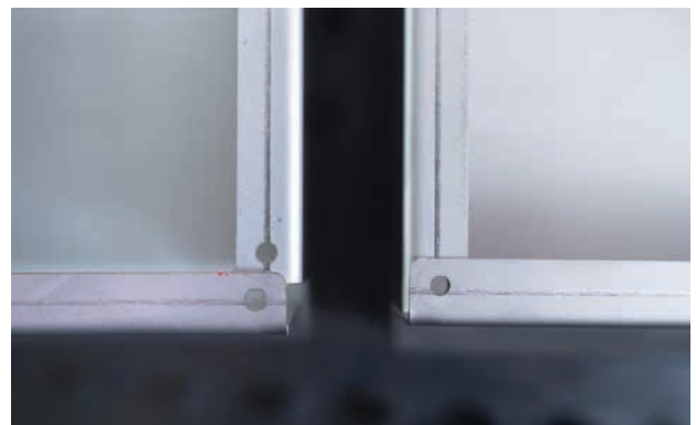
Example and details of a bent panel without corrections (left) and with corrections imported from the TMDDB (right)
