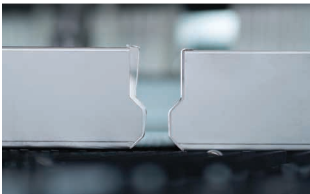
Example and details of a bent panel without corrections (left) and with corrections imported from the TMDDB (right)
