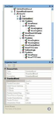
The sequence of programmed operations (loading, bending, unloading, etc.) may be collected in a treestructure that allows easy access to the different elements of the program with the possibility of adding or removing any operation at any time.
